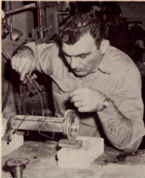
Soft soldering cooling tubes on an S-Band isolator
