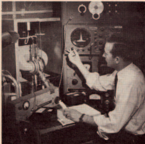
Raytheon's "Amplitron," shown under test at left center, is a new microwave power tube that increases energy output of radars. Added to the CAA air traffic control radars, for example, this tube increases the operational range by better than 50 percent.
